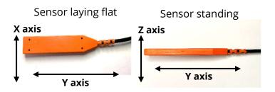
Note: The Y axis is always the direction of the cable.
