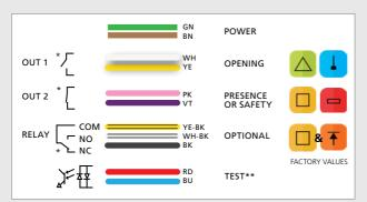
Connect the wires. The output functions can be configured if necessary, see p. 17.
