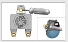
Screw the mounting bracket on the wall. You can also install the sensor directly without using the mounting bracket.
