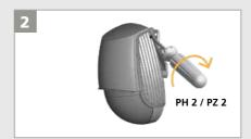
Lock the cover by turning the lock screw clockwise.
