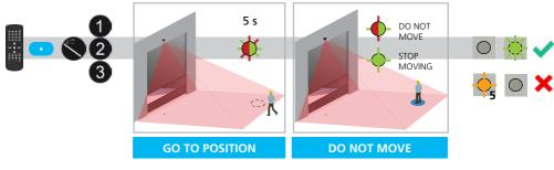
Launch a pull cord teach-in by remote control. You can create 3 different pull cords. Go to the position where you want to activate the door by a virtual pull cord.
