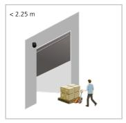
The door opens partially (motion detection - out 1)
