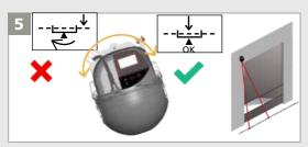
Rotate the sensor in order to align the centre of the detection field with the centre of the door using the LCD-screen. When the sensor is in the centre of the door, the position is OK.
