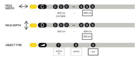
vehicle XL: detects large vehicles; rejects bicycles & small forklifts vehicle: detects all types of vehicles; rejects pedestrains any: detects all objects are detected
