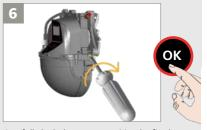
Carefully lock the sensor position by firmly fastening the angle lock screw. Make sure the red spots have not moved.
