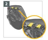
Pull the two legs on top in order to open the cover.
