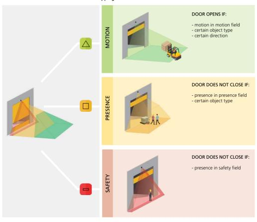
There are 4 additional functions. All detection functions can be combined to trigger a specific output (see output functions on page 16).
