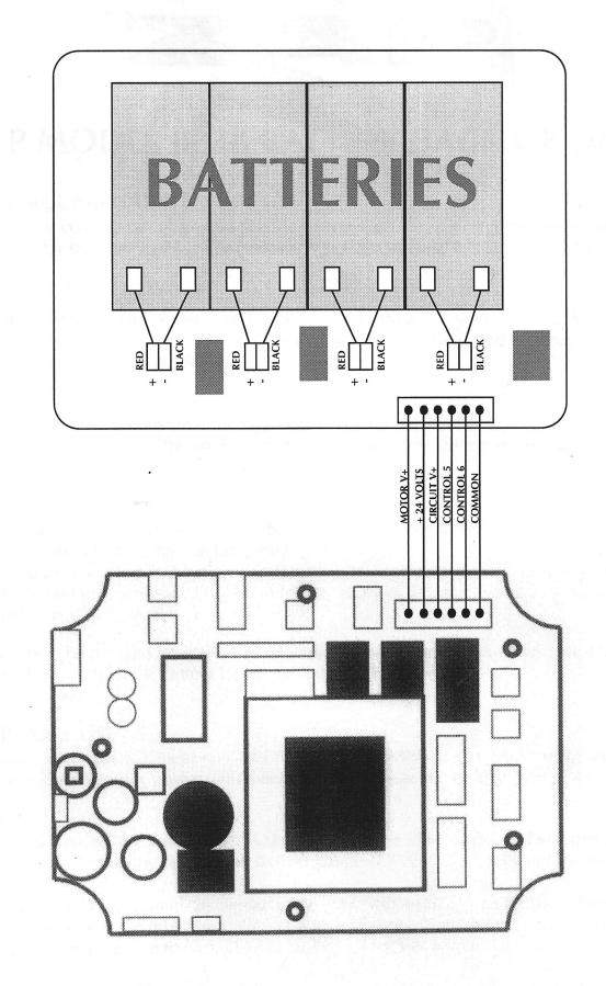
REMAINING FOUR CABLES MUST BE AT LEAST 0.5 MM SQ FOR 8800:MOTOR V + AND COMMON WIRES MUST BE AT LEAST 2.0 MM SQ CABLE FOR 800: MOTOR V + AND COMMON WIRES MUST BE AT LEAST 1.5 MM SQ CABLE
